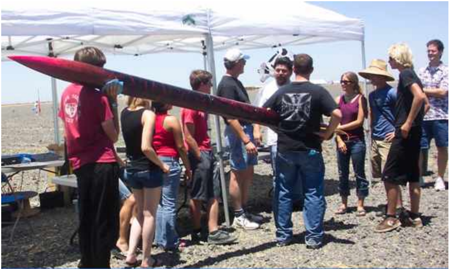
Creston Aeronautics High School students flew the ELIJAH on a cluster of 3 K550's.
