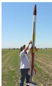
Strawberry Daiquiri on pad 41 - launch weights: 8.25 lbs (booster with J800); 14 lbs (sustainer with a J415).
