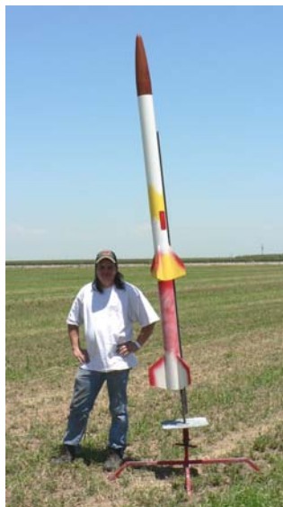
Strawberry Daiquiri on pad 41 - launch weights: 8.25 lbs (booster with J800); 14 lbs (sustainer with a J415).
