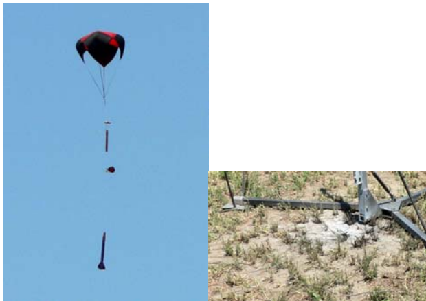
Minor scorching and no fire at the pad following exposure to the L1420R.
