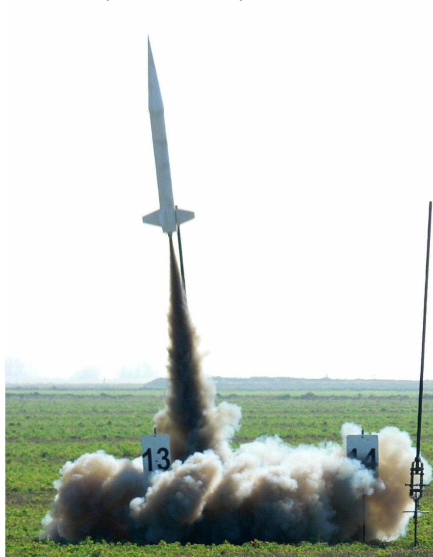
January 2008 – Steve Sawyer’s Stretch Barracuda on an H238T to 2000 ft. ART2 for dual deploy.
